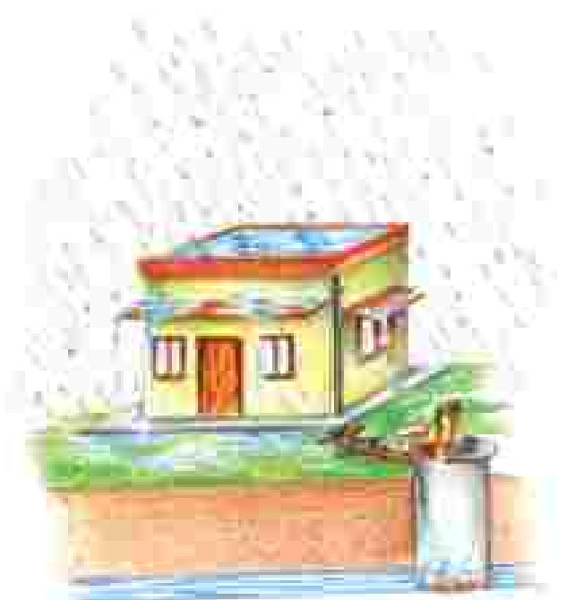
(b) Recharge through Abandoned Dugwell
